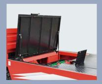
Repair, maintenance and replacement of th battery are convenient and fast, and it is suitable to continuous work
