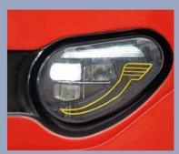
LED headlight has the head light and dipped light functions. The front turn light utilizes the latest stream light technology.
